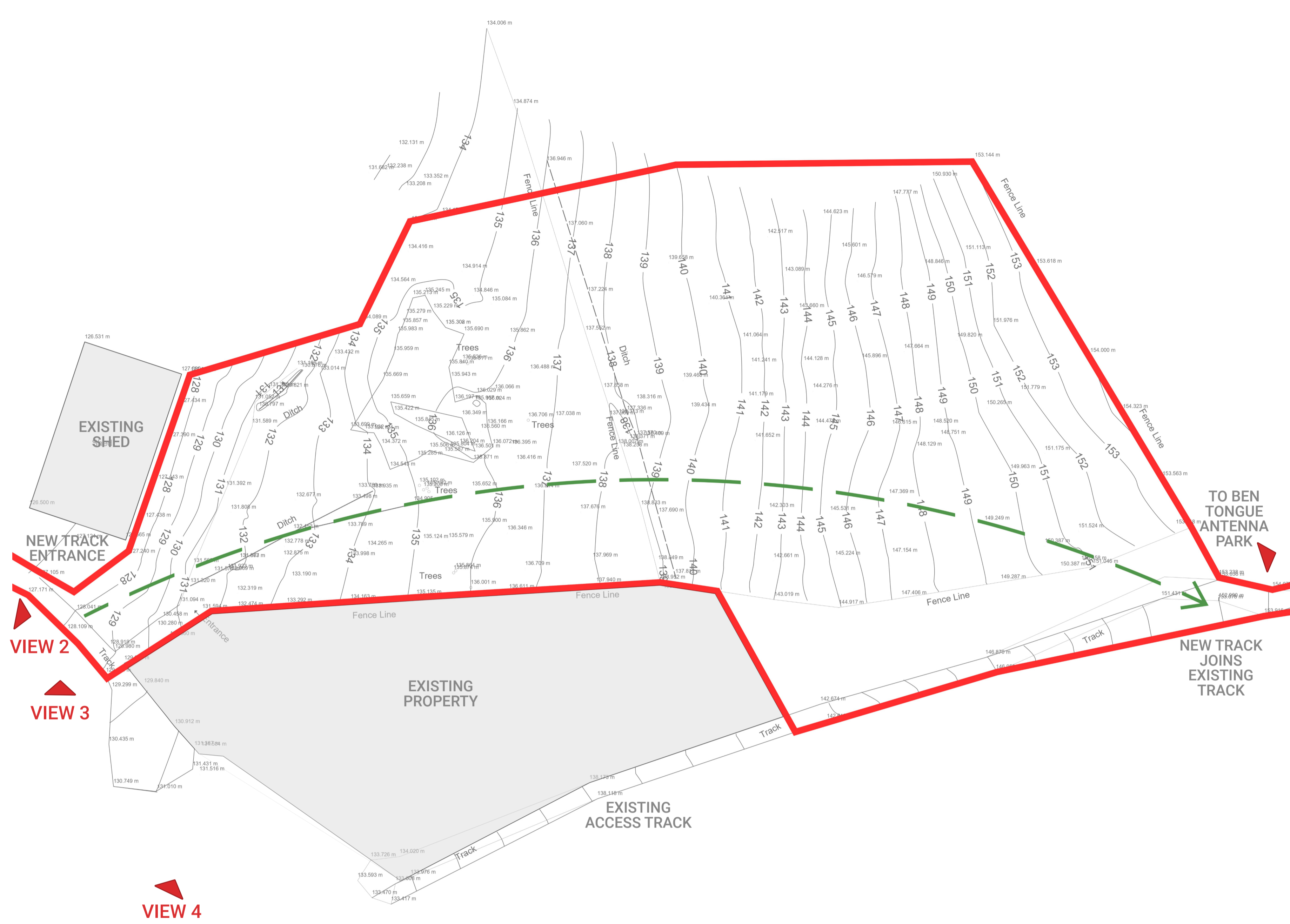
SITE PLAN - PROPOSED ACCESS TRACK AT BASE OF BEN TONGUE — SITE BOUNDARY - - - PROPOSED ACCESS TRACK - EXACT ROUTE TBC
