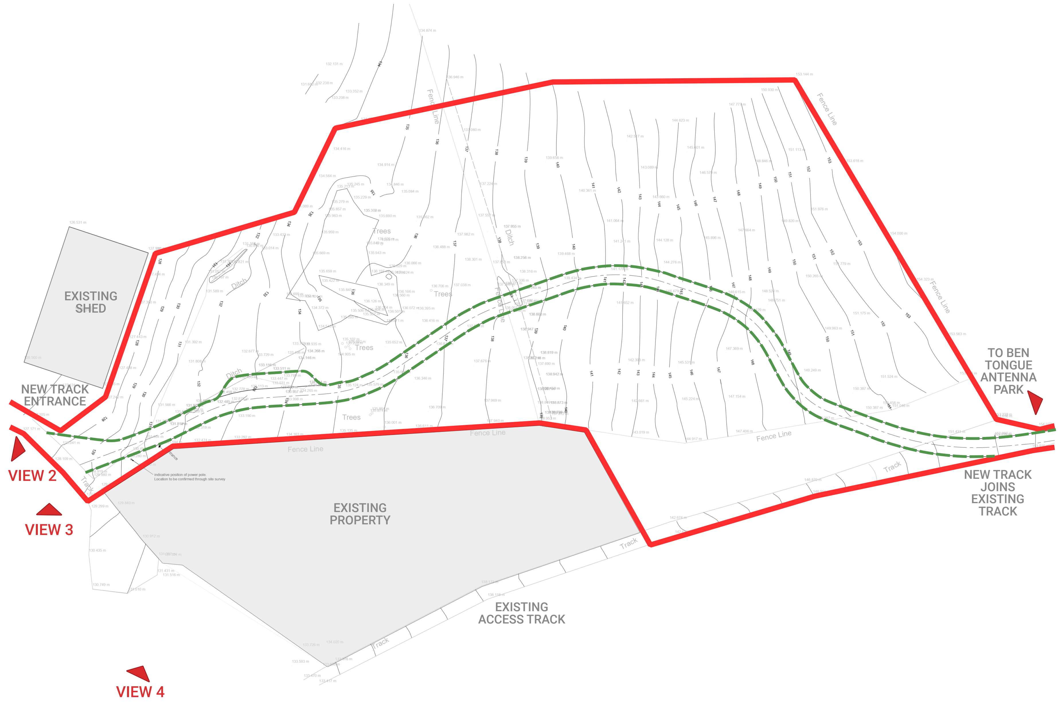
SITE PLAN - PROPOSED ACCESS TRACK AT BASE OF BEN TONGUE — SITE BOUNDARY - - - PROPOSED ACCESS TRACK
